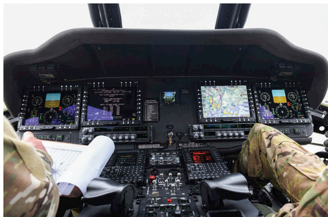
After: The digital cockpit of a UH-60V.
