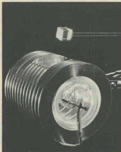
Synthetic ruby crystal (top) is the "heart" of electronic device called a laser. Ruby reradiates in a sharp beam the light absorbed from random waves emitted by light source below.
