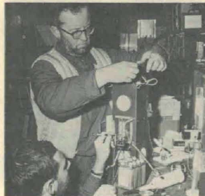
John A. Brown and Emmett J. Pybus work on hygrometer in antarctic shop.
