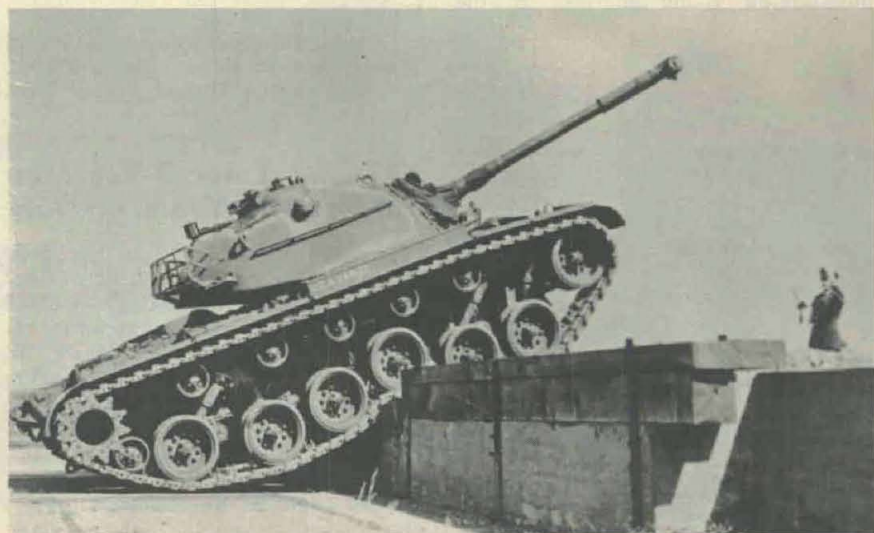
Medium tank scales 40-inch wall in one of many tests conducted by Army Ordnance Development and Proof Services for wheel and tracked vehicles at Aberdeen Proving Ground, Md., to determine combat equipment capability.
