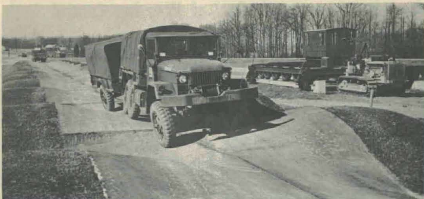
"Frame twister" road tests an Army truck at Aberdeen Munson test course.
