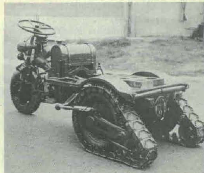
This Mountain Vehicle was designed by Italian Technical Corps for transport of weapons, ammunition, materiel.
