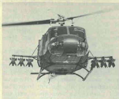
Capable of penetrating heavy tanks, SS-11 wire-guided missile carried here was developed by France under Mutual Weapons Development Program.
