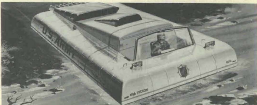
Designed to skim about a foot above land or water at speeds up to 50 m.p.h., the Ectijet experimental air car, 20 x 10 feet, is being built for U.S. Army evaluation by The Martin Co., Orlando, Fla.
