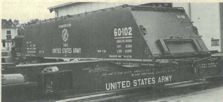
Army warhead section transporter van is swiveled on shock-reducing turntable to permit offloading from flatcar for highway movement.
