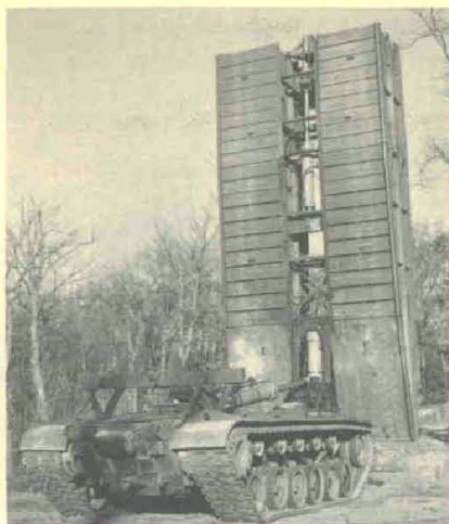
Armored Vehicle Launched "scissors" bridge; 3 new launch cylinders shown.
