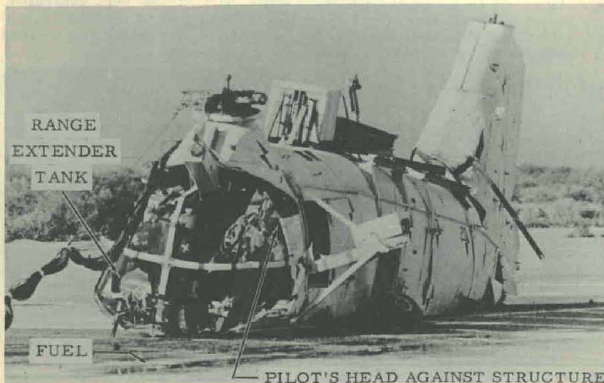
Dropped 28 feet by a crane traveling 30 m.p.h., H-25 Piasecki Helicopter remained relatively intact, sustaining but little deformation of the fuselage.
