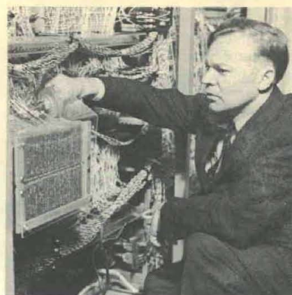
John G. Gregory, engineer in charge of the computer development at BRL, examines the 4,096-word, high-speed magnetic core storage (memory) unit.
