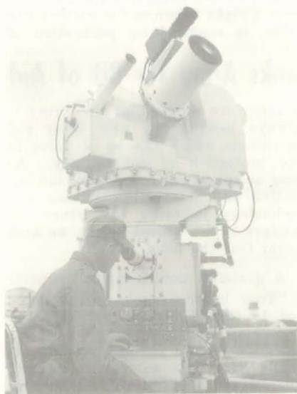
This electro-optical system known as "PIM" tracks and records flights of missiles, satellites and space vehicles with phenomenal accuracy.
