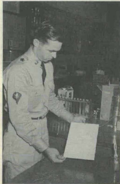
Sp/4 E. O. Harrington checks reaction of organic stripper in removing paint or plastic from test panel.
