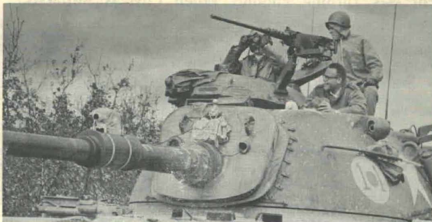
Camera (16 mm.), mounted on M-68 gun, acquires target in Friedberg training maneuvers. Shown aboard the M60 tank are the tank commander, the Army timer who stop-watched acquisition performance, and RAC observer.
