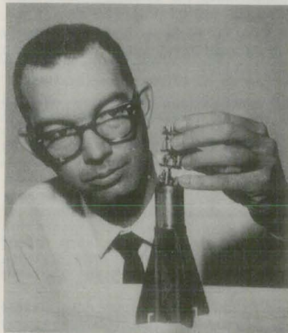
Claude A. Steffey, WSMR design engineer, fits 3-ounce, 4-channel radio into fin assembly of a Loki Dart rocket. A miniature battery is located at the base of the fins. L-shaped cuts in fins form a perfect antenna.
