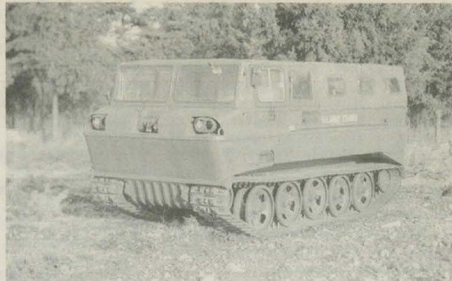
Ordnance Corps' M-116 one-ton amphibious cargo carrier.
