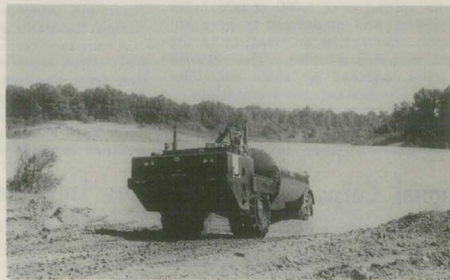
GOER emerges from water in off-road mobility tests.
