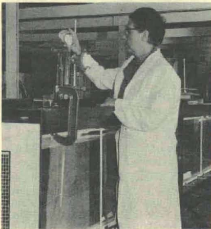
Gabrielle Asset loads a dispenser with crystals which are then introduced into the wind tunnel for observations on airflow and the mechanical, electrical and optical properties of the aerosol particles under test.
