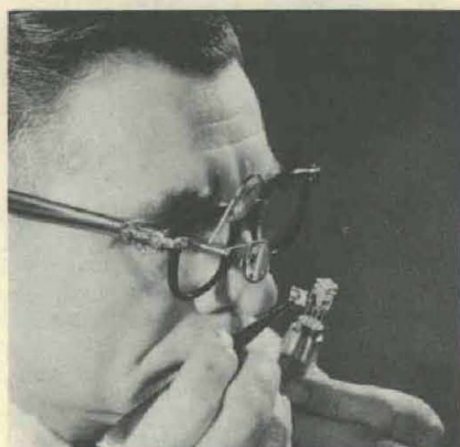
Edmund Malecki delicately adds etched "wafer" diode to micromodule already comprised of another diode, three transistors and inductor. The micromodule shown can do work of nine regular electronic components.
