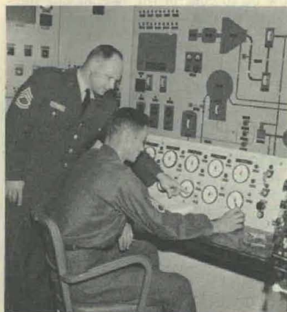
Student operator receives instruction at control console of nuclear power plant simulator at Fort Belvoir, Va.
