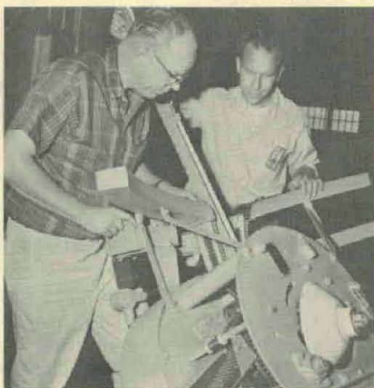
Joseph Palmer (left) and Jay Wilson, equipment designers who did basic research, developed specifications and performed evaluation tests, demonstrate 7.62mm. linking and delinking machine at Toole Army Depot.
