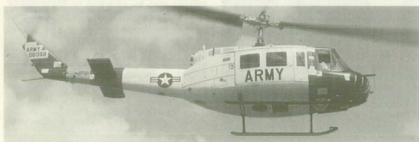
YUH-1D Iroquois prepares for U.S. Army tests in Alaska after completing Air Force tests in temperatures ranging from -65° to 125° F.
