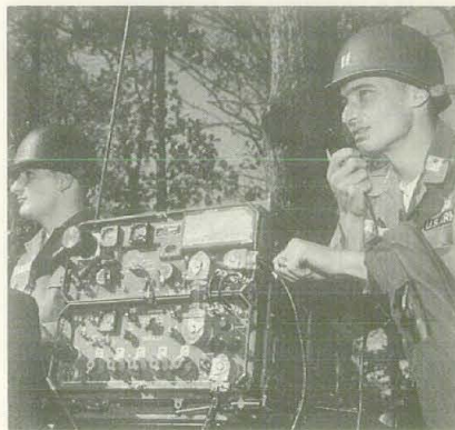
MIGHTY JEEP RADIO — "Angry-106," termed the first jeep set capable of spanning the globe, is used in combat for distances up to 50 miles.
