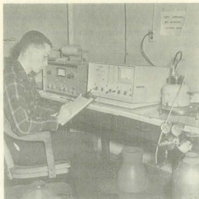
Daryl Hatfield, APG Nuclear Applications Section, takes readings from a decade scaler on sample of tools used in handling radioactive material.
