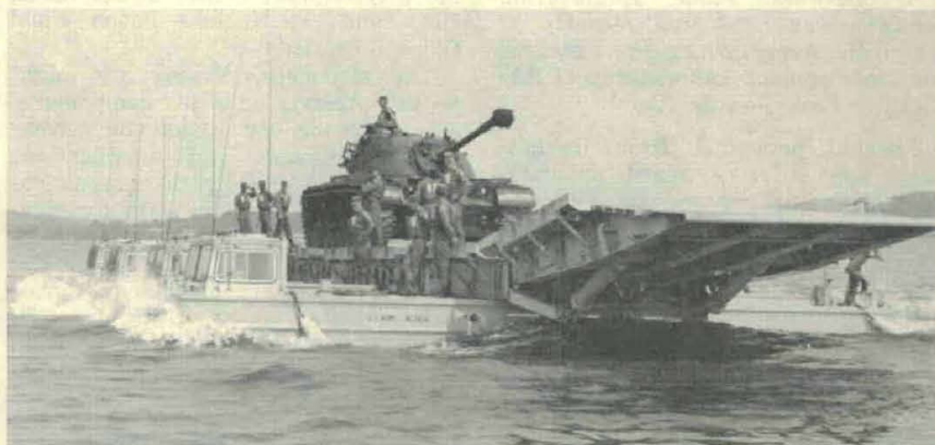
MOBILE FLOATING ASSAULT FERRY, designed by USAERDL, hauls a 47-ton tank across the Potomac River at a speed of 8½ miles per hour. The transporter can travel overland at speeds up to 35 miles per hour.
