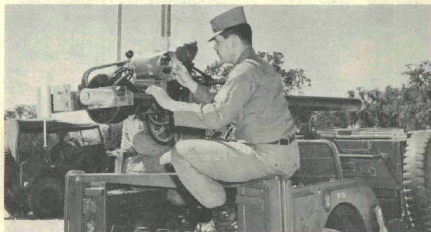
Gunner loads paper round of "ammunition" into 106 mm. recoilless rifle control unit to "ready" Hit-Kill Indicator for "firing" at the U.S. Army Combat Development Command's Experimentation Center, Fort Ord, California.
