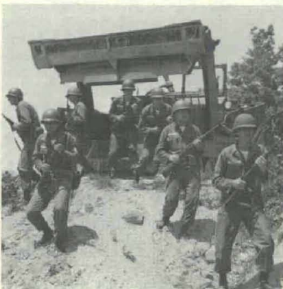
Combat construction UET, in production for the Army, performs functions of bulldozer, grader, dumptruck, scraper, prime mover, cargo carrier.
