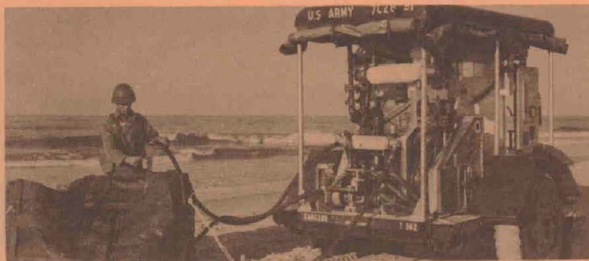
Sea Water Distillation Unit during 1,000-hour test at Daytona Beach.
