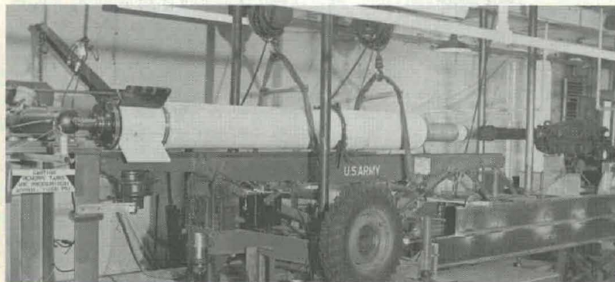
XM34, 318 mm. Rocket Launcher SSSR Spring Motor Drive, Inter-Connect Shaft Reaction Test
