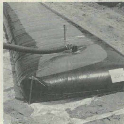
3,000-gallon, experimental, collapsible, plastic film fuel container weighs less than 35 pounds when empty. Weight includes metal fittings.
