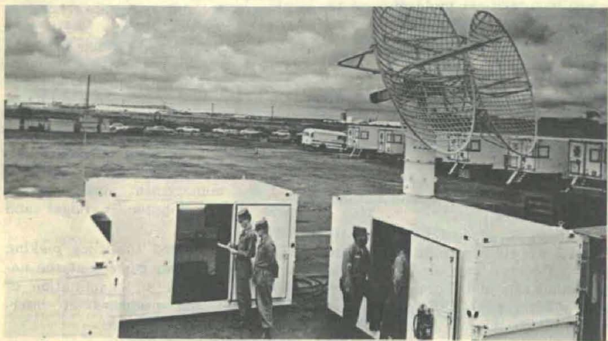
SECOR GROUND STATION units are rugged for field operations and are air-transportable. Antenna is mounted on radio frequency shelter; digitizing of the ranging and timing data is accomplished in the shelter shown in center; equipment storage and radio communications links are contained in the shelter on the left. Each station is self-sufficient with portable power, air conditioning.
