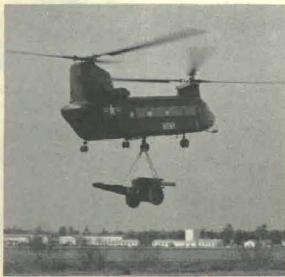
CH-47A Chinook airlifts 12,500-pound howitzer, for what is believed the first time, during service tests conducted by Service Test Division of Airborne, Electronics & Special Warfare Board.
