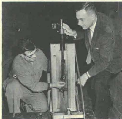
Watervliet Arsenal proof house technician Frank Mastan (left) and John Giesey examine test rig which employs a Springfield rifle to simulate firing action of a 155 mm. howitzer.
