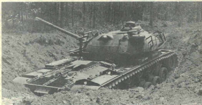
Relieved-faced cratering method of blasting barrier obstacles to stop enemy vehicles is demonstrated in tests at USAERDL, Fort Belvoir, Va.
