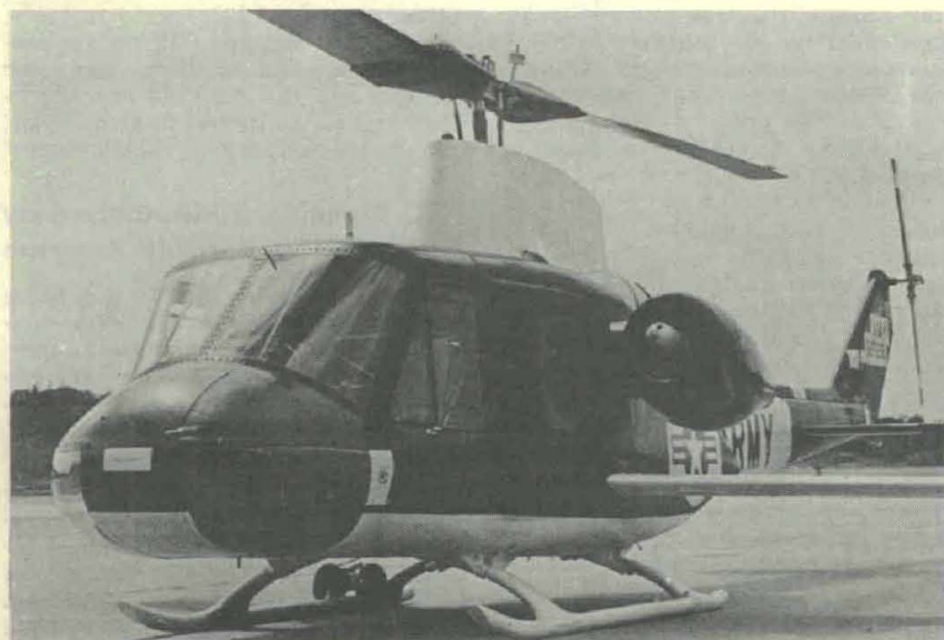
Army experimental UH-1B helicopter shown with wings and auxiliary turbojet engines. Wings were installed after recent 210 m.p.h. speed run.
