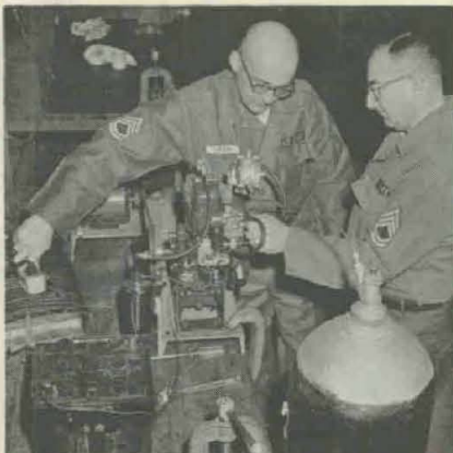
Sfc Herbert Kappel (right) regulates air flow as Sfc Frederick J. Urbin connects start-up mechanism of experimental ammonia-fueled engine.
