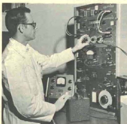
USAEPG technician Martin L. Dayton adjusts impedance measuring console, one of many devices used at the Standards and Calibration Laboratory to test Army equipment.
