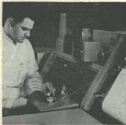
Army Missile Command scientist Robert Clem prepares sample for analysis on infrared spectrophotometer.
