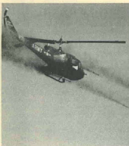
Army's UH-1B (Huey) spews forth 2.75 rockets at the rate of six per second from XM-3 subsystem recently deployed to combat areas overseas.
