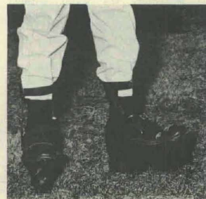
Sabot mine-clearing boot was modified by Walter Reed Biomechanical Research team to conform to position of ankle bones and feet of the soldier.
