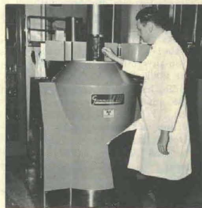
Ronald A. Sasse inserts sample into cobalt 60 gammacell 220 irradiation unit at Army Nuclear Defense Lab.
