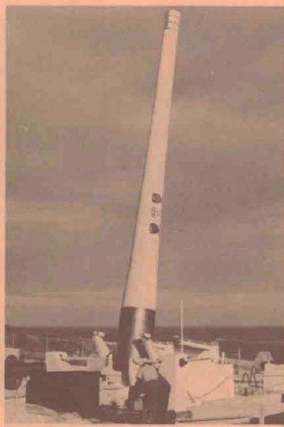
SMOOTH-BORE, 140-ton, 16-inch gun at Barbados is raised for vertical firing of projectiles in the Army's High Altitude Research Program.
