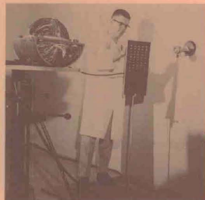
Dean Lawry, physicist, sets up missile guidance platform (left) for a test in Gama Linac exposure room in WSMR Nuclear Effects Laboratory.
