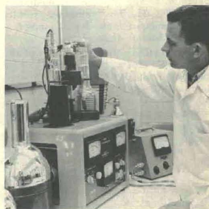
PHYSICAL METALLURGIST Julian Bynum adjusts vacuum hose on ion microscope that enables scientists at Redstone Arsenal to look at metal atoms for the first time.
