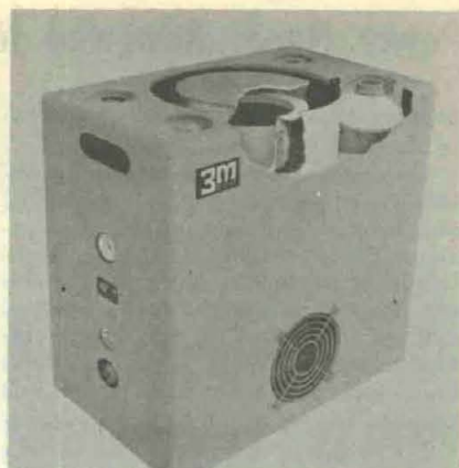
Figure 11. Proposed configuration of a flame-fired thermo-electric system.
