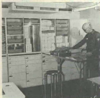
CENTRALIZED MATERIEL section in expandable shelter of MUST shows combination cabinet/shipping container concept and doors of a container being used as a work table.
