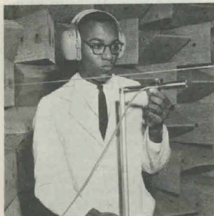
ANECHOIC ROOM helps HEL study weapon noises in a "free field" without disturbing factor of reverberation.
