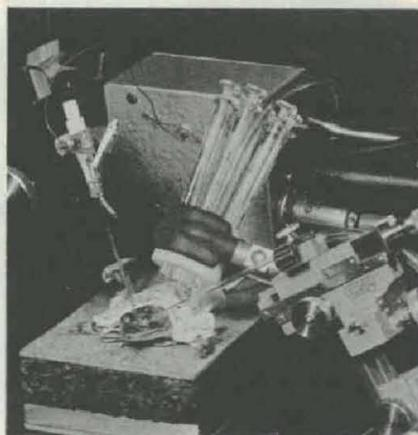
IN OLFACTORY NERVE CODING study in frog, microelectrode (left) is connected to preamplifier. Glass tube (right) passes air through nostril to supplant natural breathing. Various odors are introduced with syringe assembly (center) and patterns of nerve pulse activity are observed on oscilloscope (not shown).
