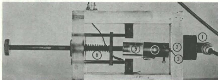
**EXPERIMENTAL ARRANGEMENT** for studying semiconductor transducer performance. A conventional transducer (1) transmits a pulse of ultrasonic energy through an aluminum plate (2) where it is picked up by the semiconductor crystal (3) mounted in a metal holder (4). A piece of lucite (5) isolates the holder from the spring mechanism (6).
