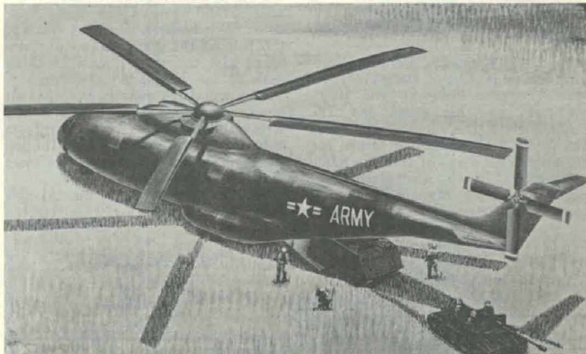
DESIGN OF A HEAVY-LIFT rotor system to enable Army helicopters to fly troops and military vehicle-weapon weightings up to 20 tons into forward combat zones is under study at the Lockheed-California Co. The giant aircraft (artist's concept above), minus cargo, is designed to travel 2,200 air-miles nonstop without refueling. Turbine-powered, it would be 111 feet long, have a rotor blade diameter of 100 feet, and be operated by a 3-man crew. The study is one of several being sponsored by the Transportation Research Command, Ft. Eustis, Va., the Army's primary aeronautical research agency.
