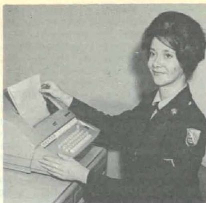
AN/FGC-80 teletypewriter, capable of operating at speeds up to 400 words per minute, is demonstrated by Pfc Judith Orr of the U.S. Army Strategic Communications Command.
