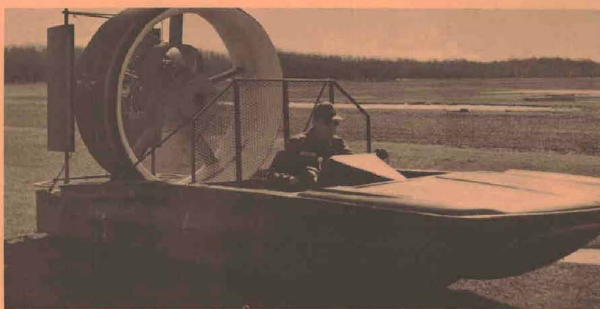
A DRY-RUN DEMONSTRATION of the Delta Reconnaissance Experimental Test Vehicle was given to about 60 members and guests of the U.S. Army Scientific Advisory Panel during a recent visit to the Army Limited War Laboratory at Aberdeen Proving Ground, Md. Especially suited for the swampy delta regions of Southeast Asia, the vehicle is capable of traveling on water, mud, rice paddies and dry turf. It is powered by a gas turbine engine that produces over 1,600 pounds of thrust.
