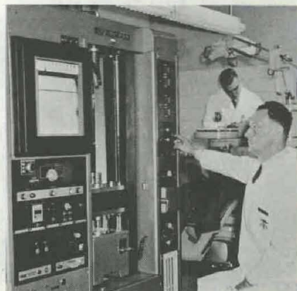
MEASURING strength of a new dental cement is Maj Simon Civjan, chief, Department of Dental Materials, USAIDR. In the background is research officer Maj Thomas V. Gardner.
