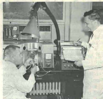
ANALYZING SAMPLES of teeth for presence of trace elements on atomic absorption spectrophotometer are Dr. Gino Battistone (seated) and Maj Francis A. San Filippo.
