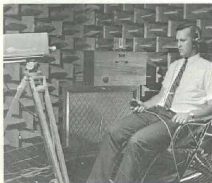
ELECTRICAL DISCHARGES are used to simulate the high intensity sounds of gun fire for psychophysiological tests conducted at USAMRL.
