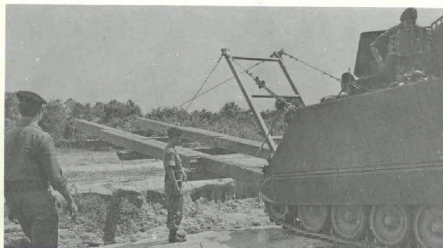
LAUNCHED by an armored personnel carrier, the 30-foot-span bridge designed by Corps of Engineers specialists for an urgent Viet Nam need can be operational (using field-available materials) in approximately 12 minutes.
