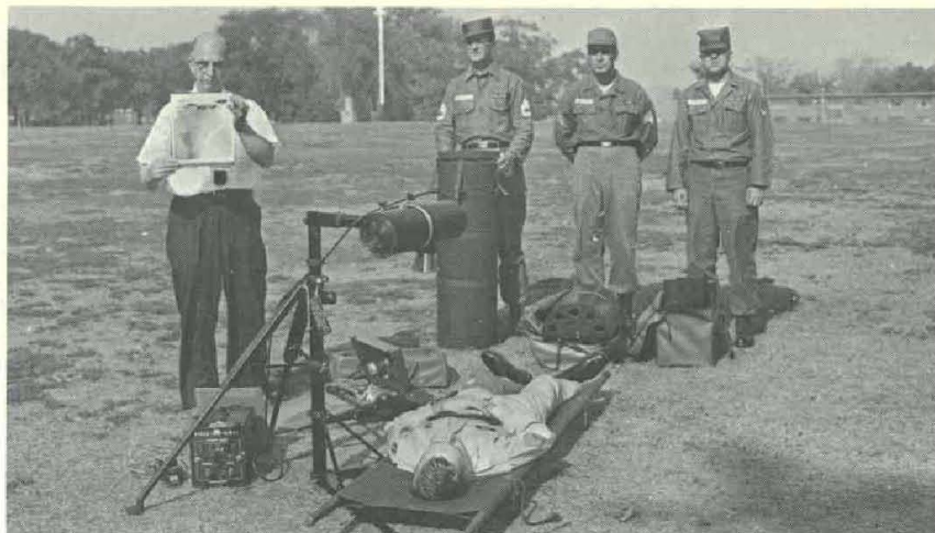
MERDL Technical Director Benjamin D. Pile demonstrates portable field X-ray unit which he designed and developed. Assisting are (standing, from left) SFC Erwin Patzke, Sgt Richard Messing and Sp-4 Dennis Sexton.
