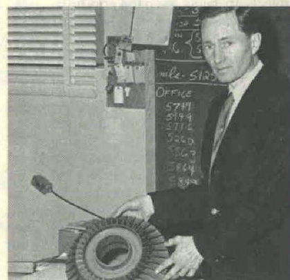
WATERVLIET ARSENAL chemist Theodore M. Pochily displays "Huey" helicopter housing treated with a protective anodized "hardcoating" and an energy-absorbing "elastomer" which retard erosion in titanium compounds.
