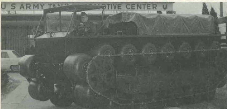
MARGINAL TERRAIN vehicle under development by the U.S. Army Tank-Automotive Center, Warren, Mich., for swamp and rice paddy travel will carry 3,000 pounds of cargo or 14 armed personnel and a crew of two.
