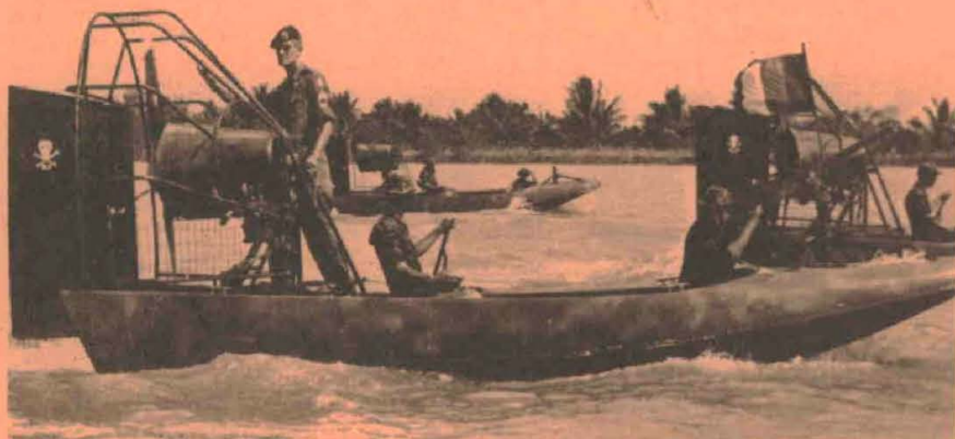
NEWCOMER to the U.S. Army Special Forces inventory is the "Aircat," an airplane-engine-powered airboat. The 180-h.p. engine can propel a crew of two and five armed infantrymen across water and swamp grass at speeds up to 48 m.p.h. A 30-caliber machinegun is mounted on the bow.
