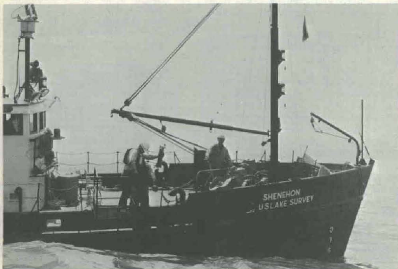
U.S. LAKE SURVEY technicians aboard the Shenehon floating research laboratory collect water samples from the Great Lakes and their overflow rivers for studies of the hydraulics and hydrology of the waters.
