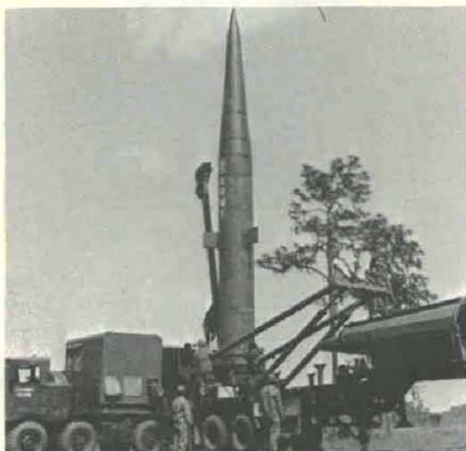
PERSHING 1-A SYSTEM features a changeover from tracks to wheels and an erector-launcher that carries the complete missile on a single carrier towed by a 5-ton M656 truck.
