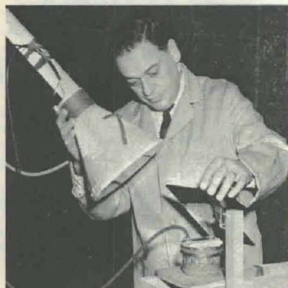
PHYSICIST Morton Sultanoff adjusts explosive flash unit and mirror before TNT charge is detonated in blast chamber at Aberdeen Proving Ground, Md.
