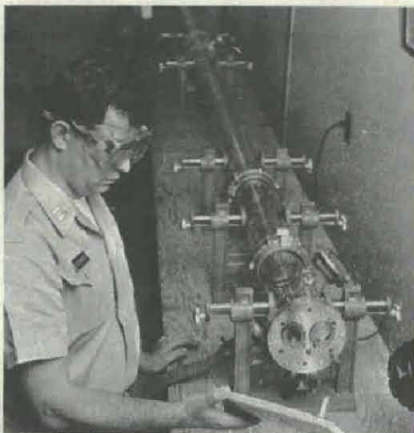
SPECTROSCOPIC TECHNIQUE adapted to improve the power and efficiency of gas lasers is demonstrated by Capt George J. Dezenberg of the U.S. Army Missile Command's R&D Directorate, Redstone Arsenal, Ala.
