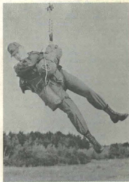
PERSONNEL/CARGO device lowers equipped trooper from hovering helicopter to area unsuitable for landing.
