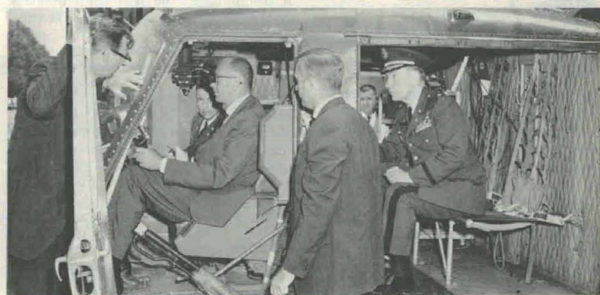
A NEW STABILIZED OPTICAL SIGHT equipped with a laser rangefinder and night-vision capabilities was unveiled recently for integration with all helicopter armament in the UH-1 series. Expected to be operational in the field soon, the sight allows the operator to track a target under all aircraft maneuvers and has been called a 100 percent improvement over what is in use. Among those present for the unveiling at Frankford Arsenal, Pa., was Howard P. Gates Jr., Office, Assistant Secretary of the Army (R&D), seated at the controls. Others, from left, are: Robert Pfeilsticker, project chief; Lt Col Lowell K. Solt, Office, Chief of R&D (OCD); Gordon Sigman, project engineer; and Lt Col David C. Money, OCD.
