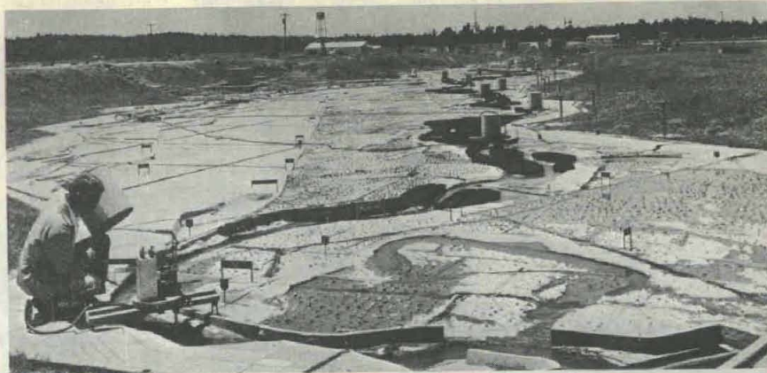
MISSISSIPPI BASIN MODEL (showing Missouri River downstream from Sioux City, Iowa) is constructed to a scale of 1:100 vertical and 1:2000 horizontal. This section of the model assisted in the flood fight of the Missouri River in 1952 by predicting where the levees would be overtopped and where they would prove adequate. The model is electrically operated from control houses shown in rear.
