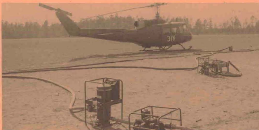
FARE, developed by the Army to service fixed- and rotary-wing aircraft under tactical conditions, was given recent engineering and service tests by U.S. Army General Equipment Test Activity, headquartered at Fort Lee, Va.
