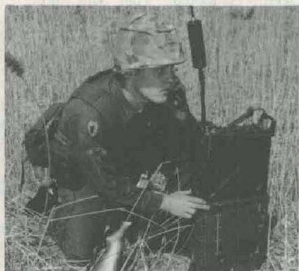
FUEL CELL undergoing tests by Army produces 30 watts of electricity for eight hours on a fuel charge the size of a pack of cigarettes.
