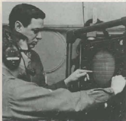
INSTRUCTOR Thomas J. Terrana assists U.S. Army Signal School student in interpreting Ground Controlled Approach display of AN/TPN-8 radar.
