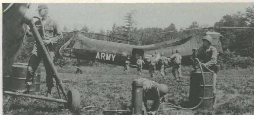
Application of 15-gpm filter/separator in helicopter refueling operations.
