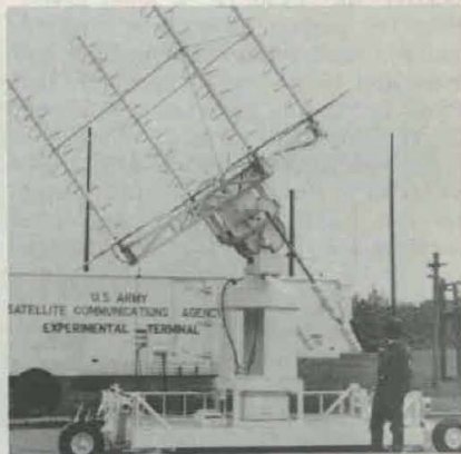
EASTT-5 terminal built for the SATCOM Agency as a "quick-fix" effort using modified equipment and vehicle.
