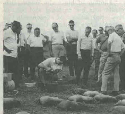
TARC MEMBERS observe as Tropic Test Center technician uses an infrared thermometer to measure surface temperatures attained by sandbags exposed to the tropical environment at the Chiva Chiva Site in the Canal Zone.
