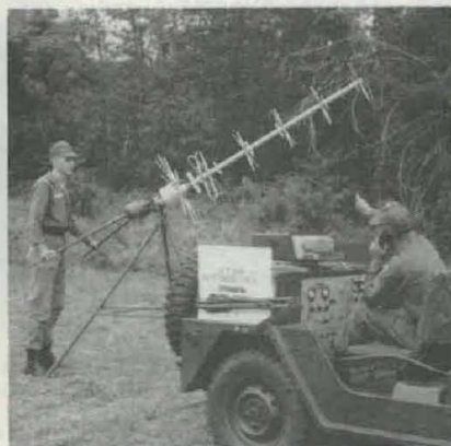
EASTT JEEP satellite communications terminal and cross-polarized yagi antenna locked on LES-6 satellite.
