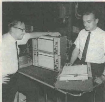
CHROMACORDER DEVELOPERS Paul Kisatsky (left) and Louis Szabo display major parts of new instrument that instantaneously measures and records the true color of burning flares. Both are employed in the Pyrotechnics Laboratory, Feltman Research Lab.
