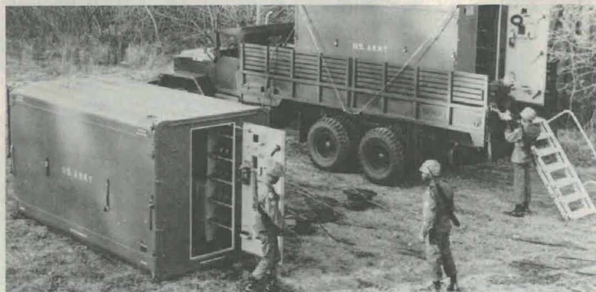
LAND COMBAT SUPPORT SYSTEM is designed to test automatically components of Army missile systems. One shelter contains test equipment, the other serves as a repair area for the Shillelah, Lance, TOW and Dragon systems.
