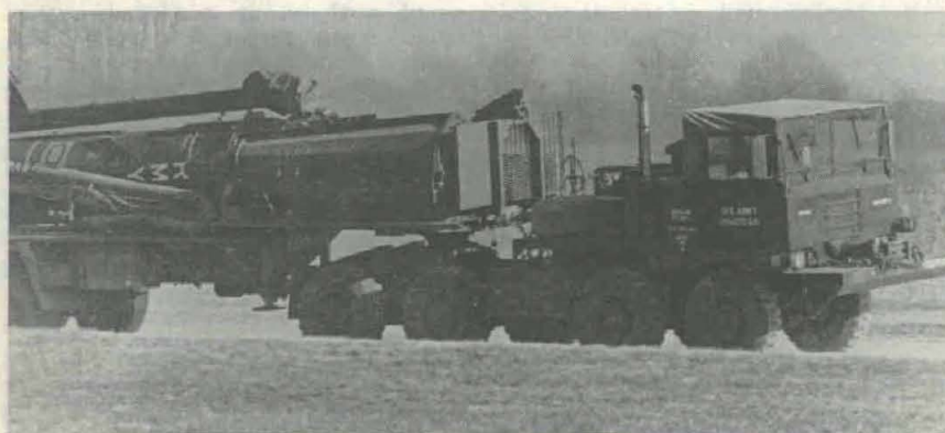
SECOND GENERATION Pershing 1A missile system, converted from tracks to wheels and equipped with many state-of-the-art improvements, is destined to replace tracked version currently deployed in support of NATO forces.
