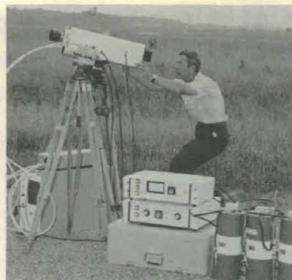
INNOVATOR Stanley M. Keen adjusts microflash system he helped develop to stop photographically an in-flight projectile's image in daylight.
