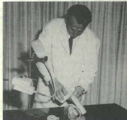
Fig. 2. CASTING caval rings, tubes, and ventricular assist pumps from the USAMBRL elastomer latex for use in testing thromboresistance qualities.
