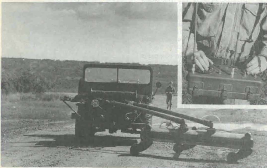
EQUIPPED WITH REMOTE CONTROL UNIT (inset), driver walks behind truck-mounted mine detector during field test of system developed by contract.
