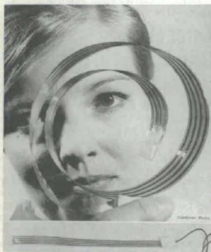
"SELF-ERECTABLE" unit, one of several built by Goodyear Aerospace to find a practical application for Nitinol, consists of four Nitinol wires encased in transparent plastic. When heated, the two inner wires cause the unit to coil. The outer two wires, when heated, uncoil unit to 18 inches.
