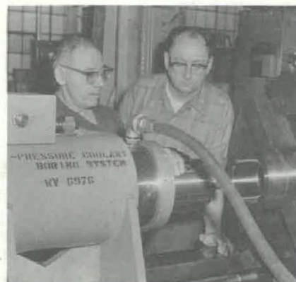
WATERVLIET machine operator William Meslanka (left) and George A. Hutson insert cutting head of new tube boring system into 155mm tube.
