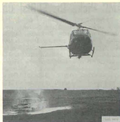
UH-1H helicopter sprays fire-suppressing foam during tests of a system designed for evacuation of persons from crashed and burning aircraft.
