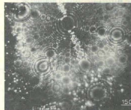
DEFECT in structure of tungsten crystal creates heart-shaped facet, upper left (magnification 1,000,000x).
