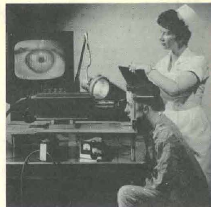
PUPIL SIZE OF EYE , sometimes a threshold effect of a drug under test, is measured by closed-circuit TV.
