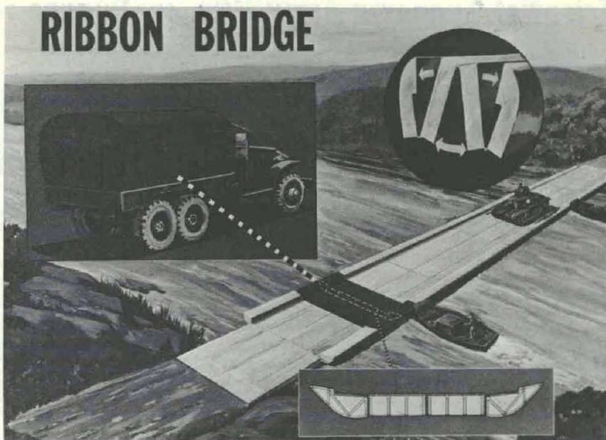
**RIBBON BRIDGE** is designed to reduce logistical problems in storing, moving, erecting and retrieving the many components of conventional pontoon bridges. Made of buoyant aluminum segments, each 22 feet long and 26 feet wide, it can be erected rapidly in lengths up to 400 feet and has a load-bearing capacity up to 60 tons.
