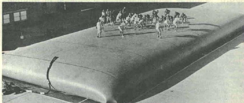
**STORAGE TANK** for 27,000 gallons of fuel is displayed in the form of one of the world's most unusual gridirons. Made of nylon coated with polyurethane, it is the largest of a family of self-supporting "pillow" tanks developed to provide mobile combat forces with unit that can be quickly erected and disassembled.
