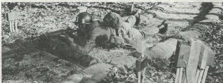
PHOTOCELLS and pressure pads monitor progress of test participants over the maneuver course at the Combat Effectiveness Test Facility, Camp Pickett, Va. Under actual conditions, the sensors that relay signals to the control and data-logging center for recording and analysis are camouflaged to avoid detection.
