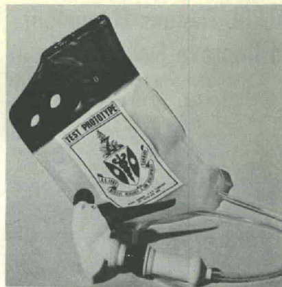
Hand-Operated Insecticide Sprayer is being developed to provide sanitation teams engaged in field operations with a control of mosquito adults, larvae, rodents, houseflies and other insect pests.
