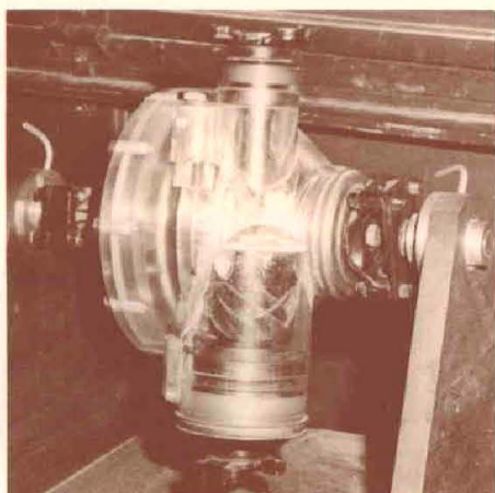
WORKING MODEL of M51 jeep differential, fabricated and machined from a clear plastic material to permit viewing of all parts when used as a training aid.
