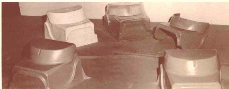
PARTS formed from high-impact styrene and finished product (top-right), a hood for training pilots in instrument flying, sometimes called a blind-flying hood.
