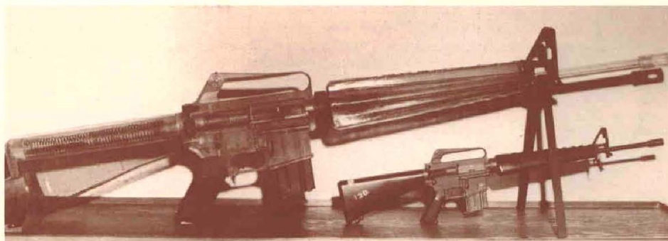
M16 rifle and plastic working model (2:1-scale) fabricated by vacuum forming.
