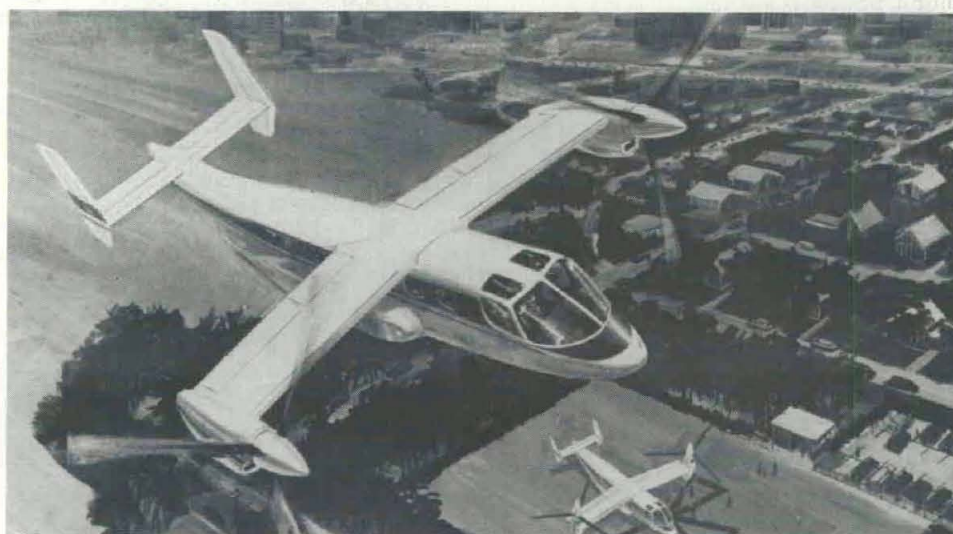
TILT-ROTOR VTOL (Vertical Take-Off and Landing) aircraft (artist's concept) is being developed by Bell Helicopter Co., under a joint contract, for the U.S. Army Air Mobility R&D Laboratory and NASA. The scheduled prototype completion date is early 1976.
