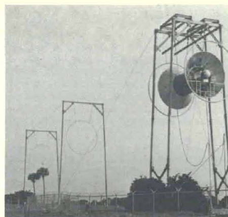
TEMPS as deployed for EMP testing at the AUTOVON switching center at Polk City, FL, extended over about 984 feet.
