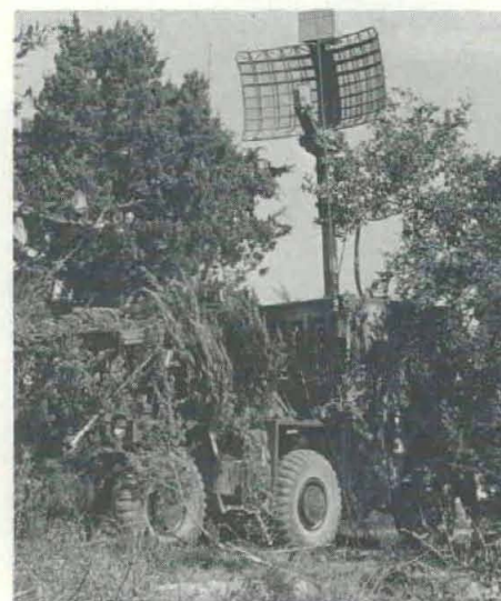
CAMOUFLAGED FAAR leaves only the radar antenna as evidence of its presence as it disperses information to individual Target Alert Data Display Sets (TADDS) operated by gunnery units in the field.
