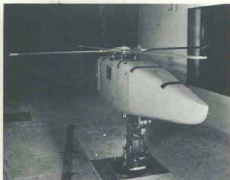
Test of hingeless rotor with all-electronic feedback control system in wind tunnel.
