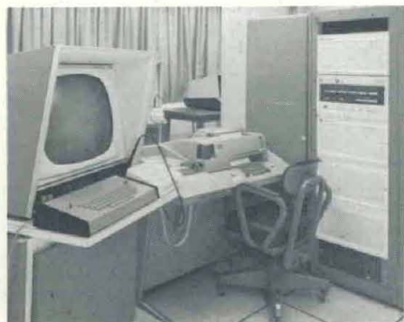
INTERACTIVE GRAPHIC DISPLAY SYSTEM showing (from left) graphics display with keyboard and light pen, teletype for input/output, data communication, and Varian 620-F11 Mini-computer. Included in the system (not shown) are an electrostatic printer-plotter, disc storage, and the paper-tape punch and card reader.
