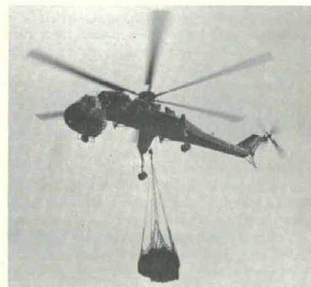
NATO Inventory Net (loaded), manufactured in Great Britain, is airlifted by a CH-54B Flying Crane, during an evaluation at Yuma Proving Ground, AZ.
