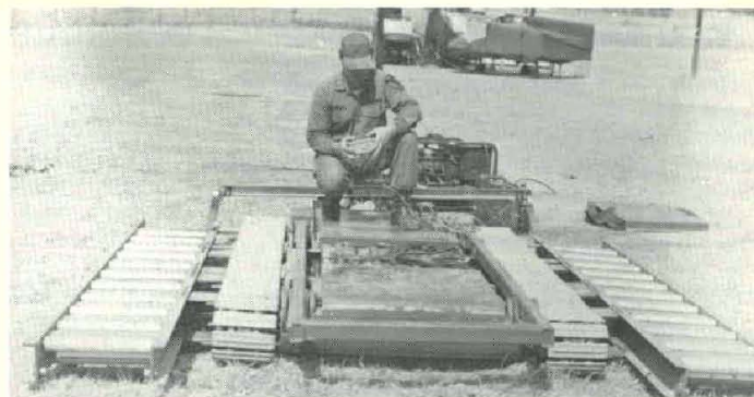
HELICOPTER TRANSPORTER is a battery-powered, tracked vehicle with a winch to pull helicopter onto roller conveyors.
