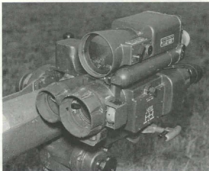
CANDIDATE Night Sight for TOW Weapon System (Texas Instruments Co. Model)
