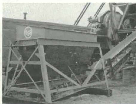
Fig. 2. VIBRATING SHAKER passes fibers onto conveyor belt at a rate of about 800 pounds per minute. The fibers were dumped into shaker by a front-end loader.
