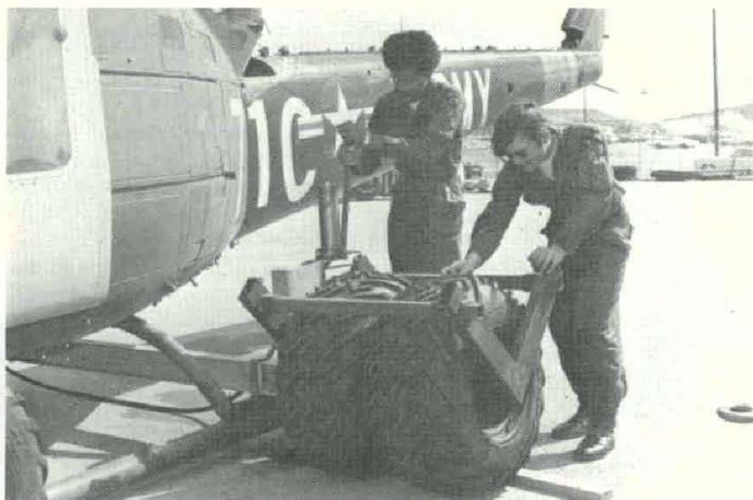
FIELD WHEELS , equipped with a manual or electric hydraulic system, allow a helicopter to be lifted over rocks or other small obstacles. Unserviceable helicopter hulks are used in the tests.
