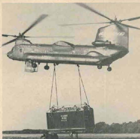
MODEL 347 Fly-by-Wire flying testbed lifting a MILVAN standard container.
