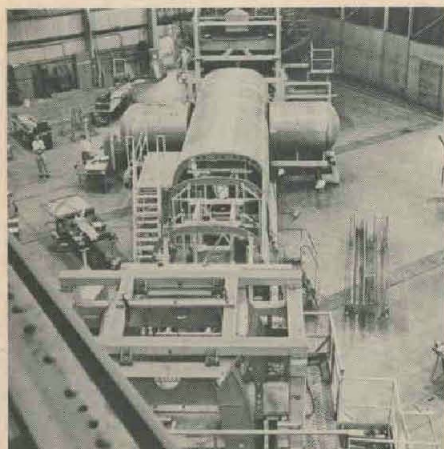
HLH Prototype fuselage assembly at Boeing Vertol plant in Philadelphia, PA.
