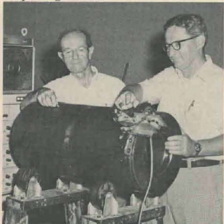
James J. Miller (r.) and Donald C. Winters displays their patented device that has improved ultrasonic testing of gun tubes.
