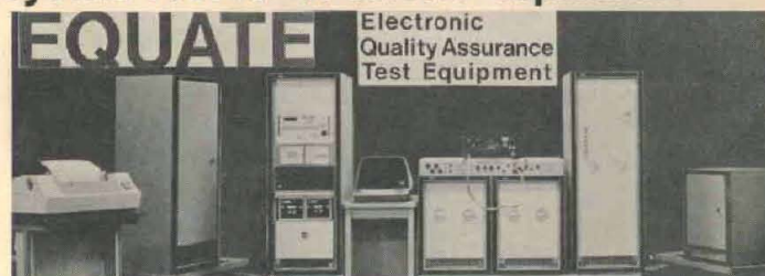
EQUATE configuration, above, includes (from left) a line printer, a d.c. power station, computer station, UUT station, r.f. station, and an a.c. power distribution station.
