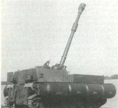
M109A1B self-propelled 155mm howitzer, with inflated flotation kit, prepares to enter Chesapeake Bay waters for APG evaluation.
