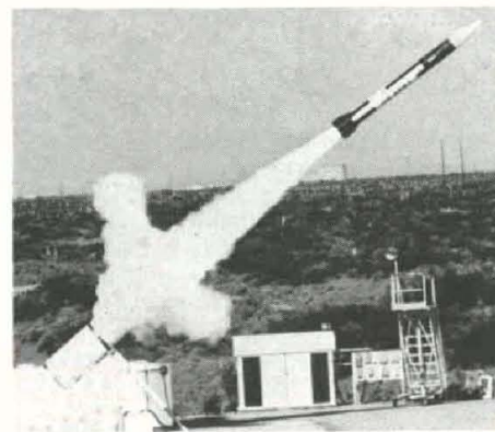
SAM-D , single-stage solid propellant missile, with latest technology in propulsion, guidance, electronics and armament, clears launching rig during test firing at WSMR.
