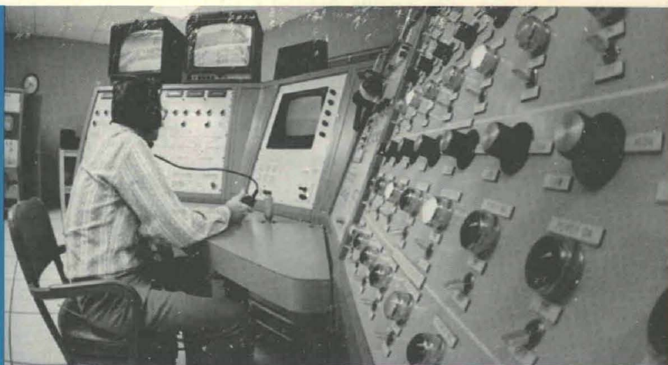
Control console for terrain model at Missile Command Advanced Simulation Center.
