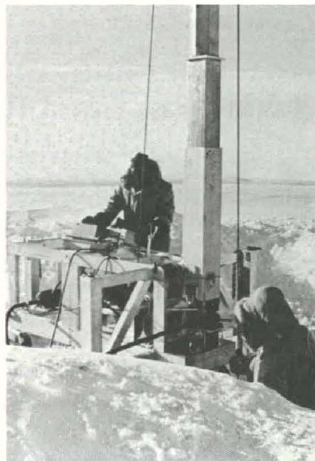
CRREL lightweight mechanical shallow drill was first tested on the Greenland ice sheet and was proven in Antarctica during the 1974-75 austral summer R&D program.
