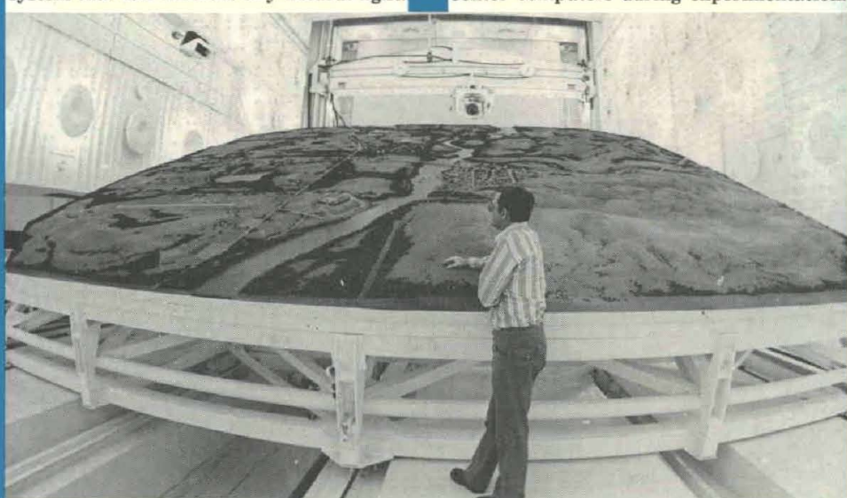
MISSILES can be tested for ability to acquire, track and destroy enemy targets under day or night conditions at the electro-optical cell, a 1,024-square-foot moving terrain model covered with miniature deserts, mountains, rivers, dams, towns and military targets.
