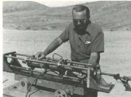
Lanyard-fired, modified .22 cal. weapon is used to simulate terminal ballistics of 30mm AP rounds of ammunition at reduced distances at the Yuma Proving Ground, AZ.
